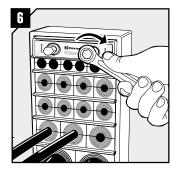
Insert the Roxtec Wedge and tighten the screws until full stop.
