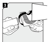
Lubricate all modules for the frame thoroughly, both the inside and the outside surfaces.
