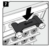
Attach the Wedge Clip to the wedge bolts to check that the wedge is properly tightened.
