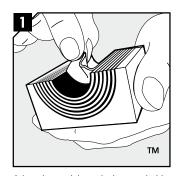
Adapt the modules, which are to hold cables or pipes, by peeling off layers until you reach the gap seen in pic. 2. The halves may not differ by more than one layer.
