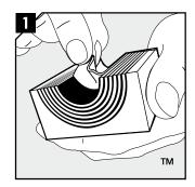
Adapt modules, which are to hold cables or pipes, by peeling off layers until you reach the gap seen in pic. 2. The halves may not differ by more than one layer.
