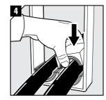
Insert the modules according to your installation plan (transit plan). It is recommended to seal cables/pipes at the bottom of the frame and put spare modules on top.
